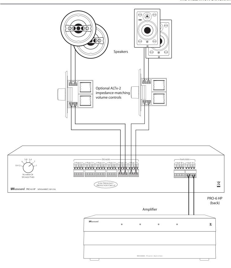
PRO speaker selector diagram showing connection of speaker and amplifier (Not to scale)
