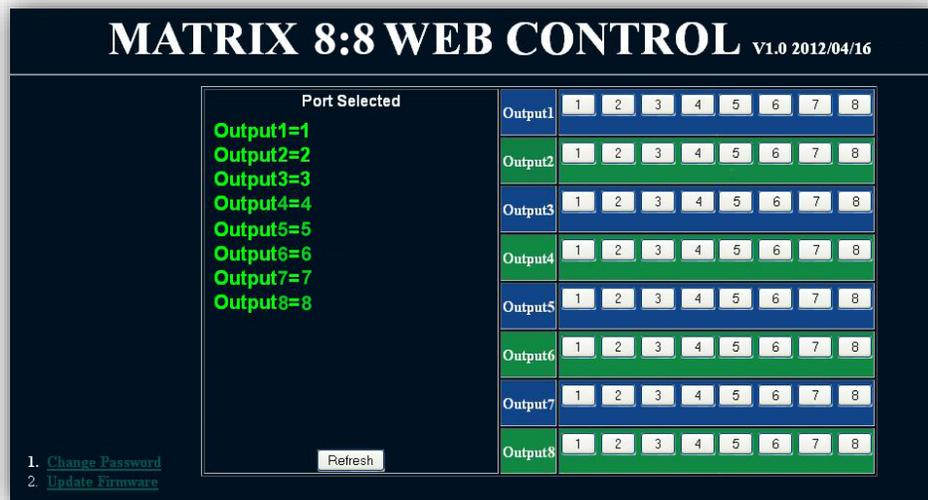
5. Clicking the buttons after each output changes the HDMI routing accordingly.
