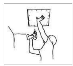
Insert the speaker, make sure there is no strain between the underlying insulation and speaker. Screw through all pre-drilled holes. The heads of the screws should penetrate about 1 mm into the panel material.
