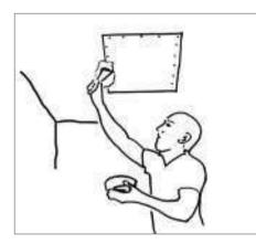
Fill in plaster, we recommand to use a flexible filler, e.g. Knauf Uniflott or Ardex 828
