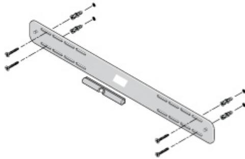
7. Fasten the PLAYBAR bracket to the wall using the screws supplied in the wall mount kit. Use the level to verify accuracy a final time, and then tighten the screws securely.
